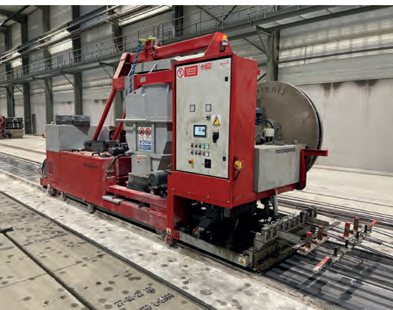
Automatic multi-function bed cleaner from Nordimpianti
