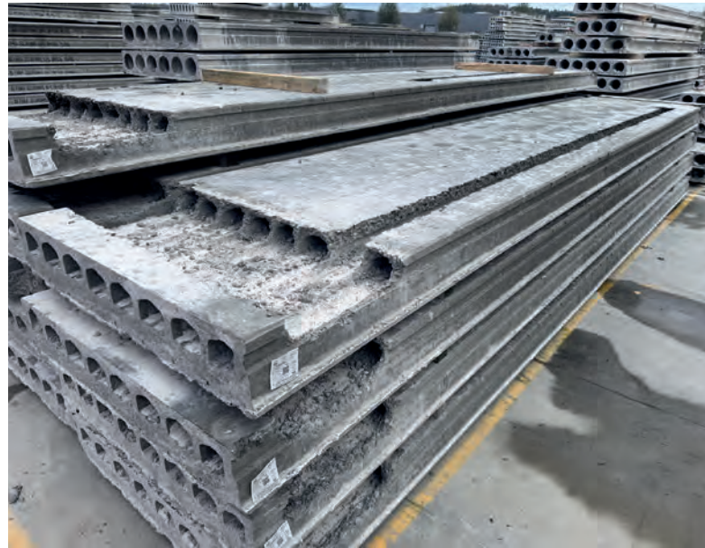
On the left: hollow core slabs with insulation, on the right: hollow core slabs with channels specific to the Dutch market
