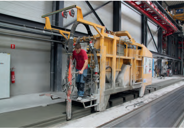
Manual Concrete Aspirator operation at the Malle factory
