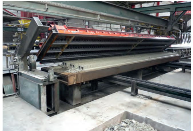
Carousel plant for non-prestressed hollow core slabs
