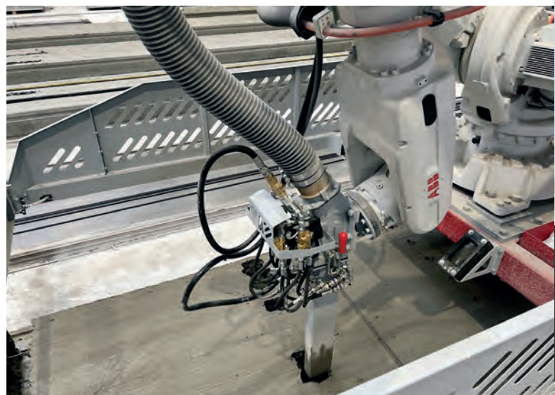
The new Automatic Concrete Aspirator developed by Nordimpianti for the Tessenderlo production plant
