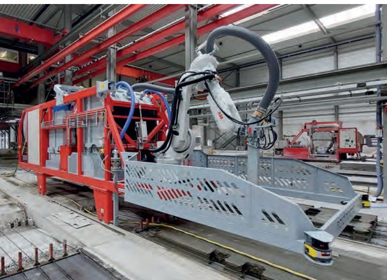
The new Automatic Concrete Aspirator developed by Nordimpianti for the Tessenderlo production plant
