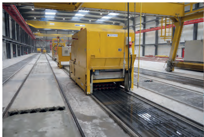
Extruder casting machine casting hollow core slabs at the Malle factory
